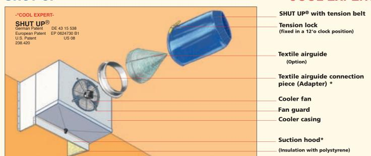
\* mounted by cooler manufacturer or by installer
